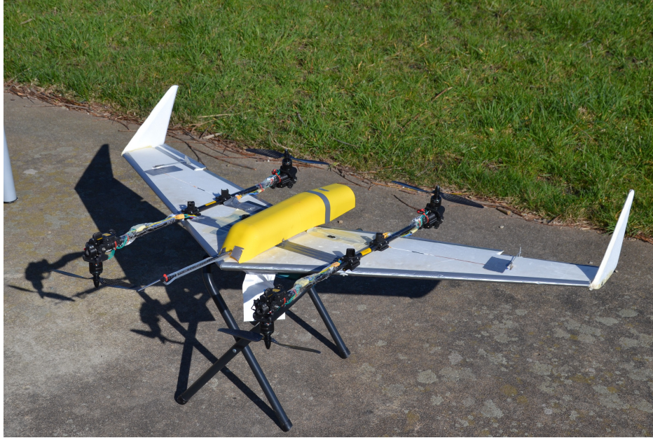
Figure 1 Dual-axis tilt-rotor quad-plane developed by Mancinelli et al. [2]. Photo courtesy of Nico Voß.
