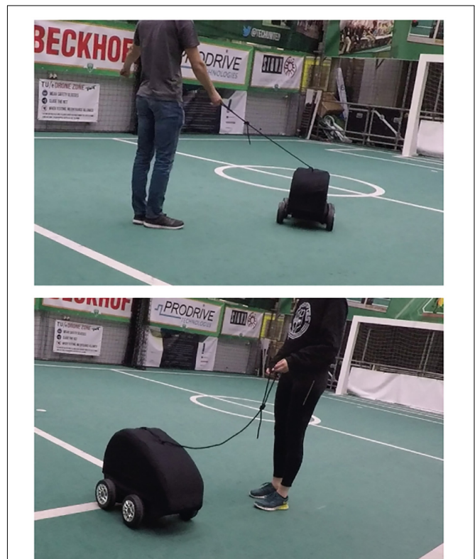
FIGURE 2 | Two participants interaction with the robot showing a situation with a stretched leash and thus in a leading role (top) and situation with a loose leash and thus a following role (bottom).
