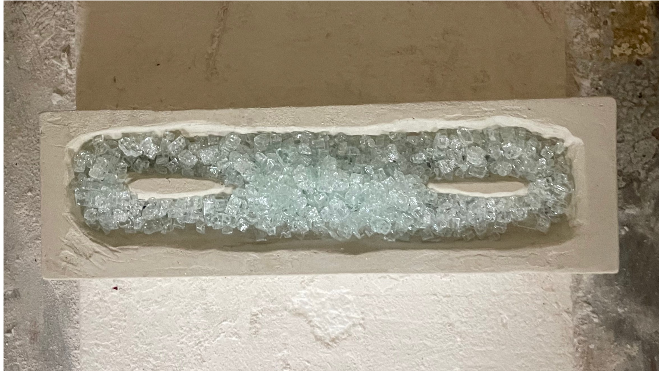
The new float glass prototype with all glass inside the mold
