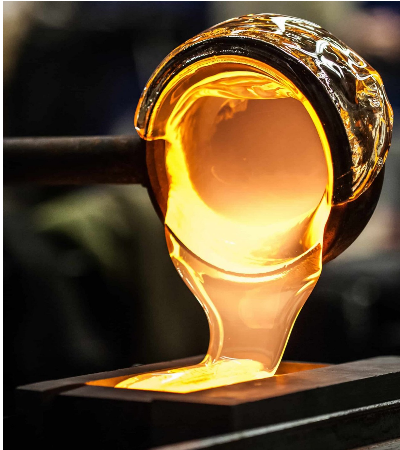
Hot forming and Kiln Castin
