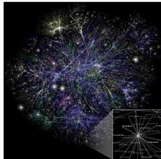
**Figure 1.2:** Visualization of IP-addresses and connections between IP-addresses connected over the internet. Color corresponds to geographical location, white being the internet backbone. The Opte Project / Barrett Lyon [CC BY-SA 4.0](https://creativecommons.org/licenses/by-sa/4.0/)
