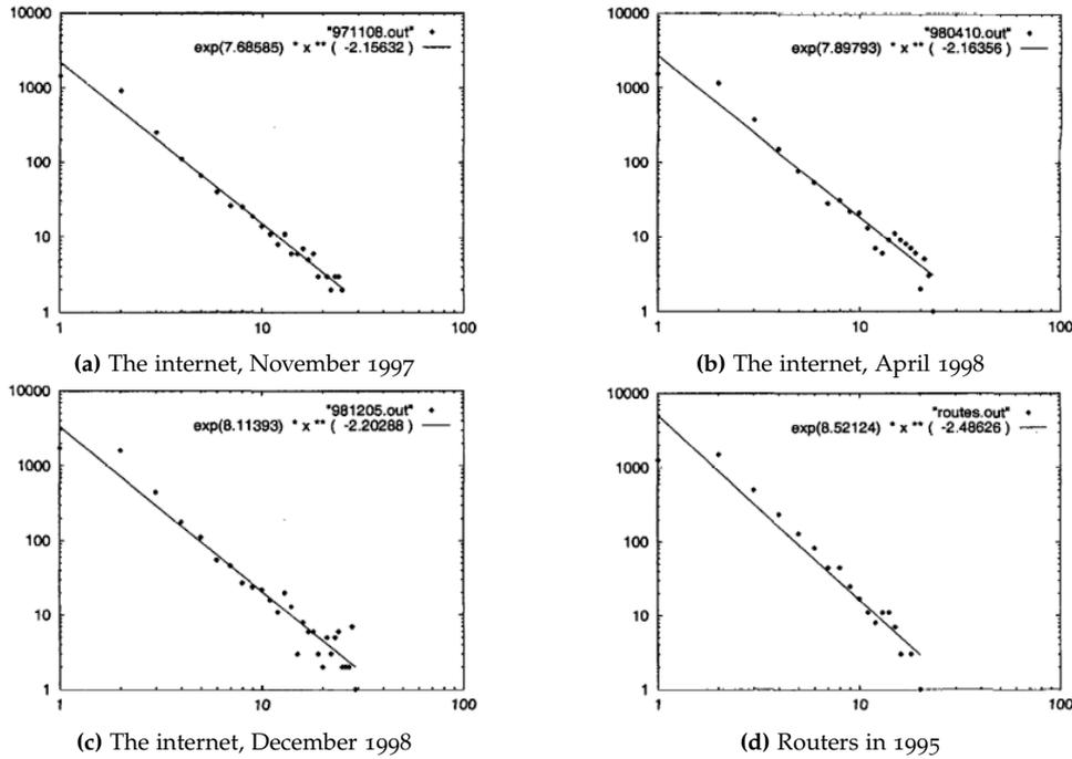
**Figure 1.3:** Four log-log plots from Faloutsos *et al.* [18], describing the relation between the log of the total degree (x-axis, described as log of the out-degree in the article) and the log of the frequency that this degree is found (y-axis). Figures 1.3a to 1.3c, describe the number of hyperlinks between domains (not discerning the sub-domains after the /) in the internet at the respective dates. Figure 1.3d, describes the connections between routers in the internet in 1995.
