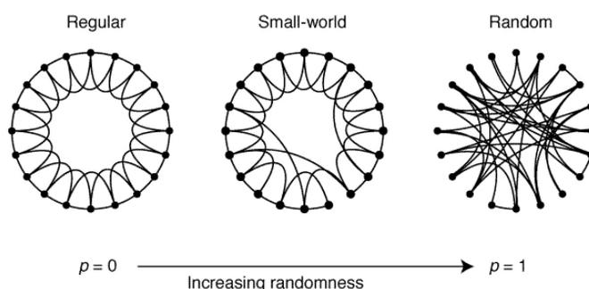
Figure 1.4: The Watts–Strogatz model [25]. Re-used with permission of publisher.
