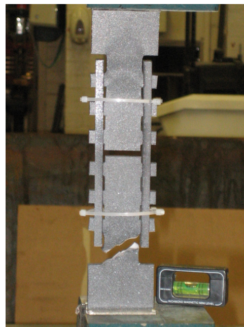
Figure 9. Failure mechanism of scaled side ISC flanges
