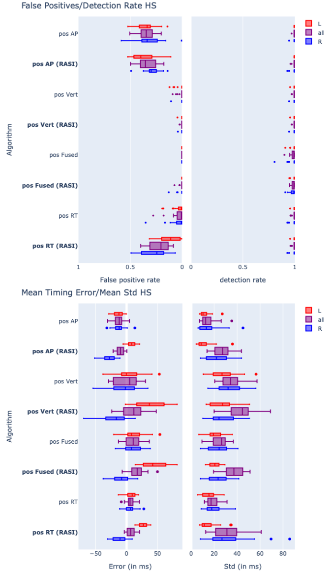
Fig. 6. Comparing the robustness of the algorithms by using a marker located further from the CoM (RASI). In the top row, the false positive rate and detection rate . The bottom row shows the mean timing error and the variance of the timing error
