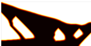
Figure 2.16: Design obtained with overhang filter using a conventional initial design. To obtain good results, starting with a fully solid design is recommended. C = 1.69C_{\text{ref}} .
