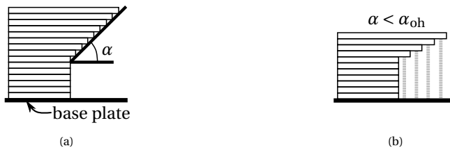
Figure 2.1: The overhang angle is defined as the angle \alpha that a down-facing surface of the combined printing layers makes with respect to the base plate (a). Down-facing surfaces below the critical overhang angle need to be supported by support pillars, indicated with gray dashed lines (b).
