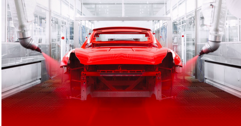
Figure 12: Ferrari's painting process [11]
