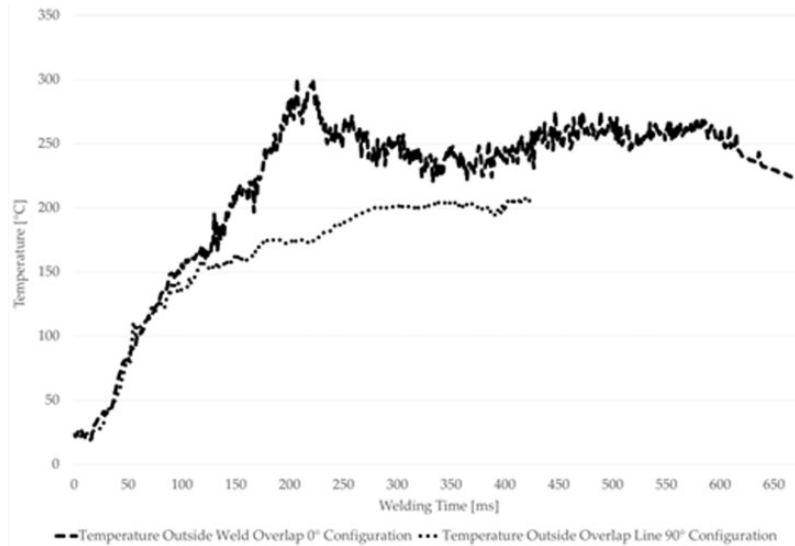
Figure 9. Temperature measurement outside the weld overlap on top of upper adherend for configuration 0° sample (solid line) and configuration 90° (dotted line). Welding performed with 86.3 \mu\text{m} amplitude, 1000 N weld force and 0.16 mm vertical displacement.
