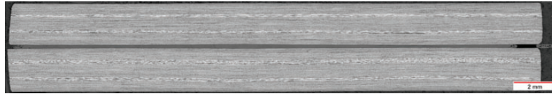
Figure 13. Transversal microscopic cross-section of samples using 30 \times 17 \text{ mm}^2 energy director. Welding parameters are 86.3 \mu\text{m} amplitude, 1000 N weld force and 0.16 mm vertical displacement. Minor resin squeeze out can be observed.
