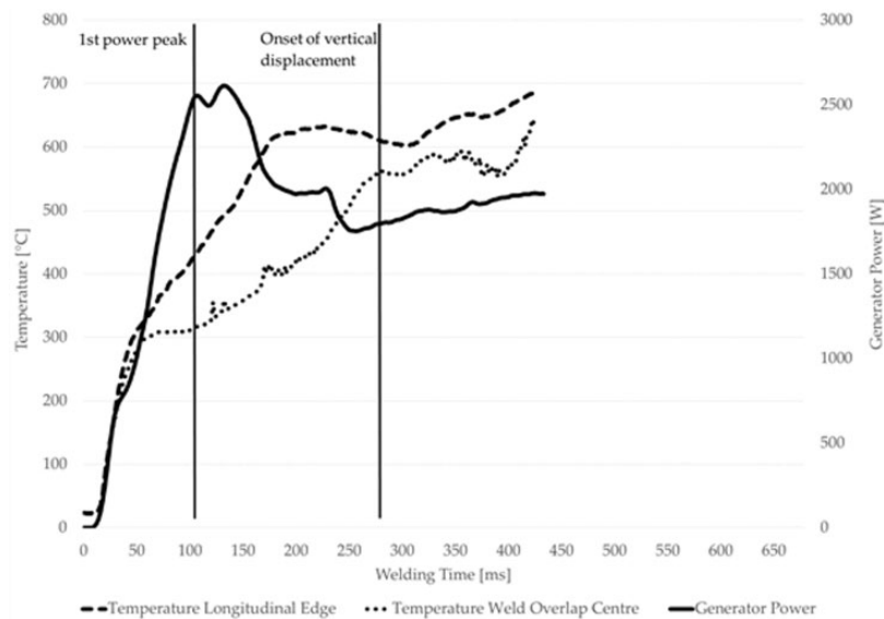
Figure 8. Temperature measurement at the weld overlap centre (dotted line) and longitudinal edge (dashed line) for configuration 90^\circ sample. Welding performed with 86.3 \mu\text{m} amplitude, 1000 N weld force and 0.16 mm vertical displacement. Vertical lines indicate 1st power peak and onset of vertical displacement.
