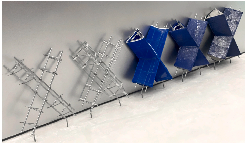
Fig. 2. A typical node of the proposed construction system during the different construction stages (from left to right): actively bent rebar cage with stirrups as gridshell falsework; plastic rebar spacers, supporting shuttering rods; flexible knit shuttering; resin impregnation for stiffening; and concrete cast integrating the falsework as stay-in-place reinforcement.
