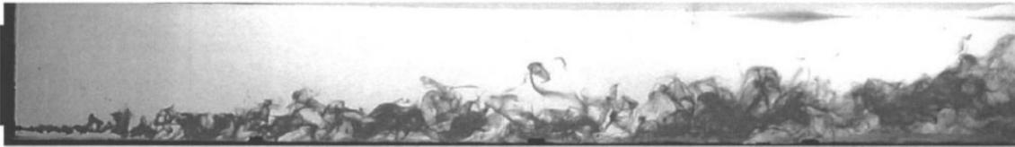
**Figure 5.1:** Laser-induced fluorescence measurements of a turbulent plume by Webster et al. [78]. The plume is released isokinetically close to the wall into a fully developed boundary layer.
