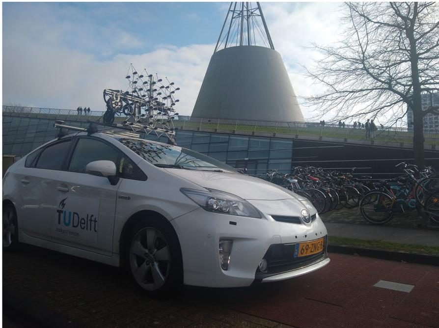
Figure 1.2: Display of the research vehicle with the mounted microphone array on the roof.
