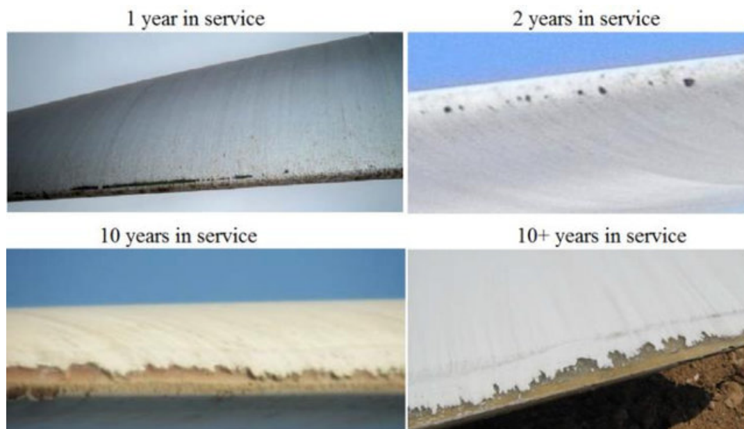
Figure 1.4: Leading edge erosion examples following different number of service years. From [29].
