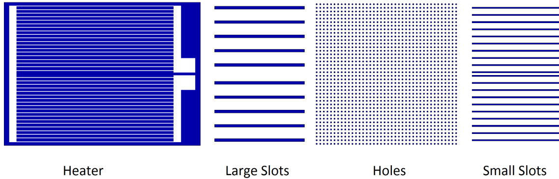
Figure 1. Masks used in the manufacturing process of the devices. The same heater mask was used in all devices, namely GLS, GH and GSS chips.
