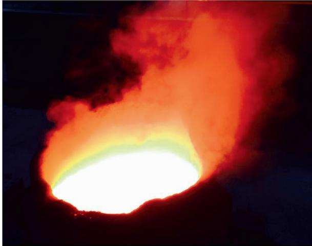
Figure 3-24. Graphite dust escaping from a hot metal ladle after slag removal.
