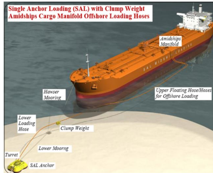
Figure 2.13: Single Anchor Loading system [55]
