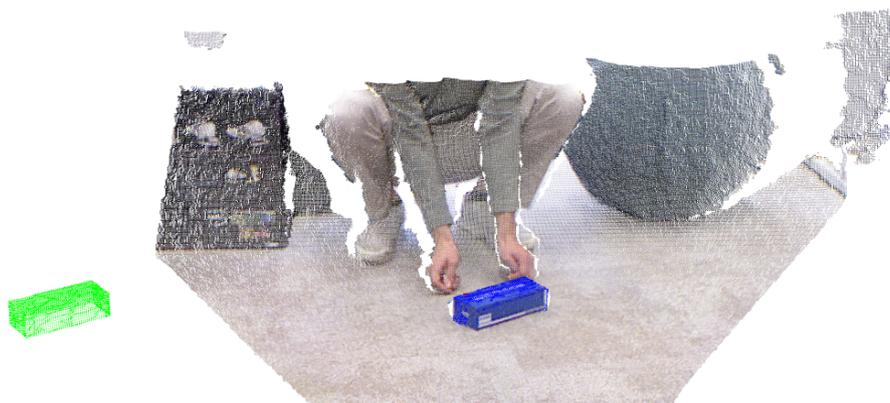
Figure 4.3: Visualization of the particle filter-based tracking algorithm. The blue points on the object represent the actual position of the object that is tracked; the green points serve as a reference to get a better idea of its behavior.
