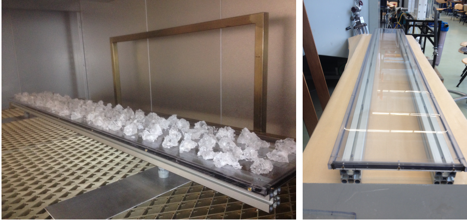
Figure 5.7: Pre- and post-heating of the coating material a) Pieces of coating material on a constructed polycarbonate plate, and b) Smooth coating layer with a homogeneous thickness, in the order of \sim 5 mm.
