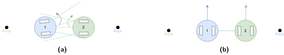
Figure 7-5: Collision avoidance. Figure 7-5a illustrates the moment the collision is detected. Figure 7-5b illustrates the movement of the robots to avoid the collision. The dashed lines represent the field of view of the proximity sensors.
