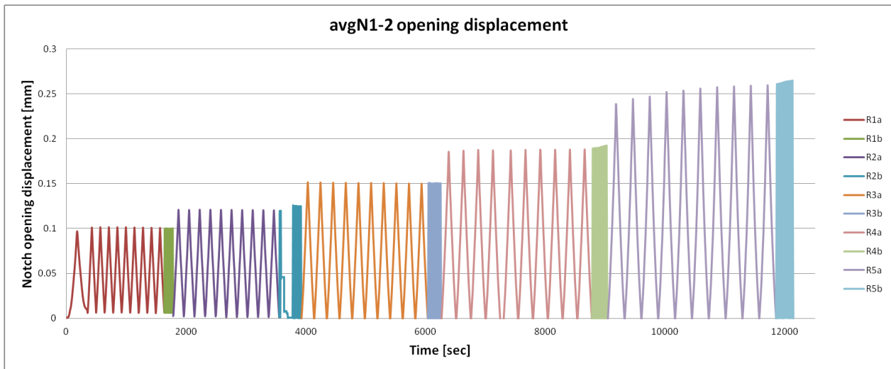
Figure 4.41. Average opening displacement of notch 1 and 2.
