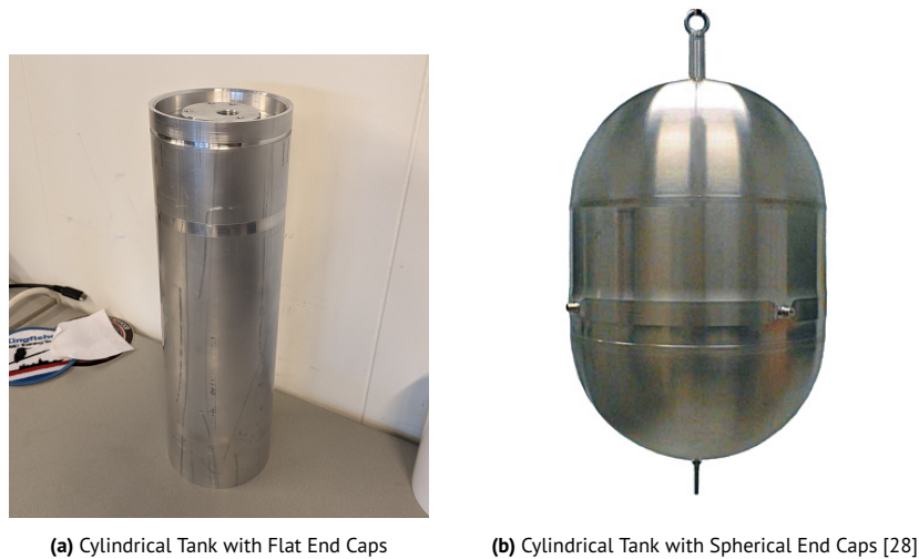
Figure 3.13: Both types of propellant tanks in the fluid tank module
