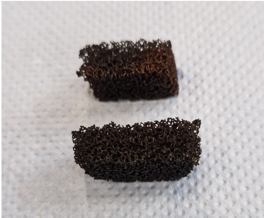
Figure 3.2: Initial Production Test Items of the Manganese-Oxide coated Nickel catalyst bed
