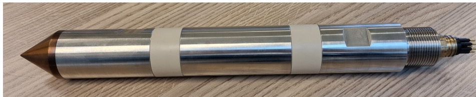
Figure 4.2.: Test probe used for the heat flow cone penetration laboratory tests.
