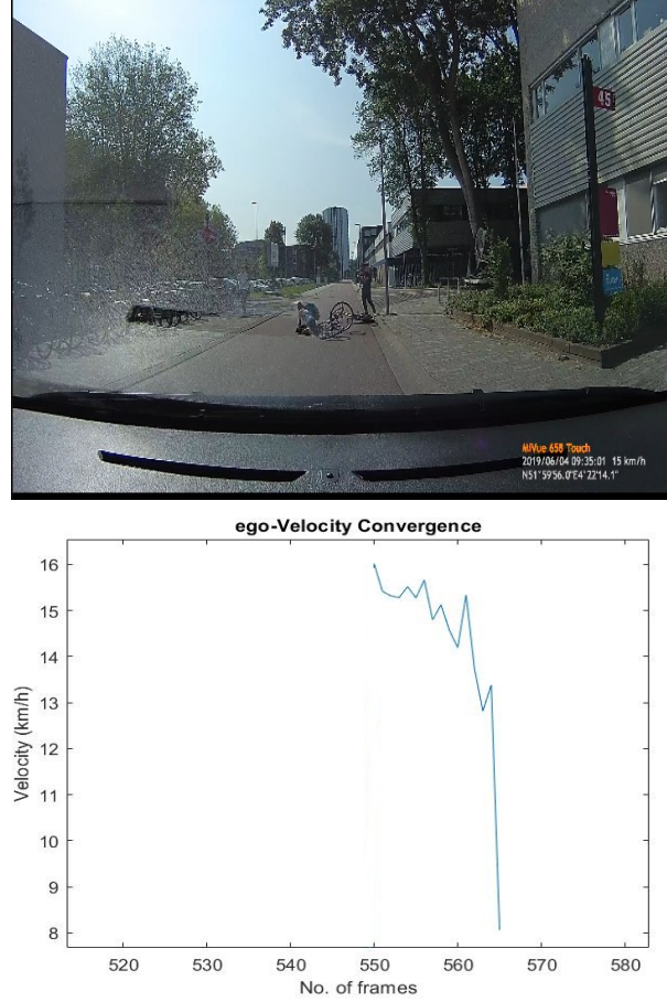
Figure 5.5: Real Measurement data 2: Validation of ego-velocity tracking
