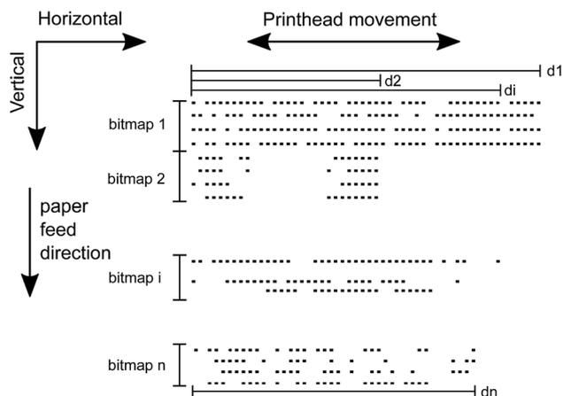
Fig. 5 To determine  $t_{\text{req}}$  for any pattern, the pattern needs to be divided into  $n$  bitmaps. In the  $i^{\text{th}}$  bitmap,  $d_i$  is the index of the rightmost droplet to dispense. The dimension of bitmap  $i$  then equals  $r \times d_i$ , where  $r$  is the number of nozzles for a particular color of the printer. To simplify the figure,  $r$  was chosen to be 4. The Epson Stylus SX235W actually has 90 black nozzles and 29 nozzles per color.
