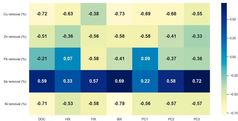
Fig. 3. Correlations between HM removal efficiency (%) and fluorescence characteristics of feed water.
