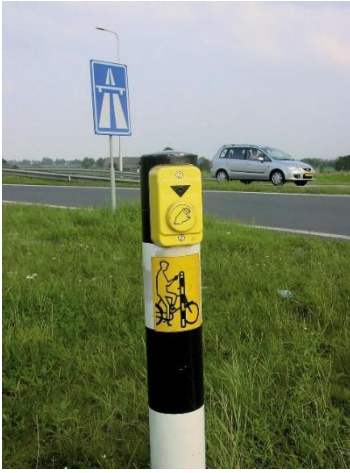
Figure 2: A inductive push button (CROW, 2014)
