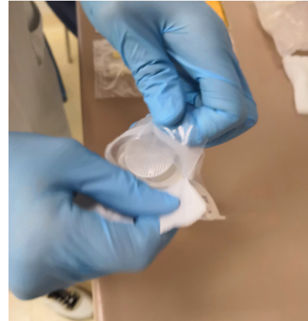
3. The packaging with syringe is opened. The syringe is taken out without touching the tip.
