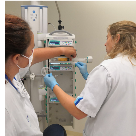
20. The syringe is placed into the pump. The pump is closed, and the display shows the type of syringe.
