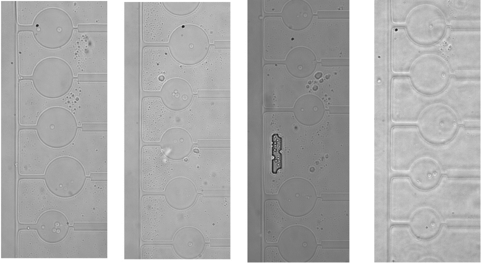
Figure S3.3: Widefield micrographs of B. subtilis spheroplasts in the microfluidic trapping chambers. Approximately 40% of the traps contain a single spheroplast.
