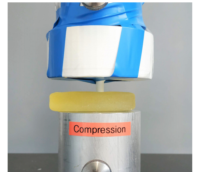
Figure 6.18. Experimental setup of the compression test 2 to evaluate the effect of the scale on the consistency.
