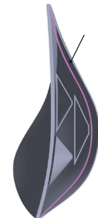
Figure 6.48. Layer of flexible material (Agilus30Clr) that separates the cones zone from the front zone.
