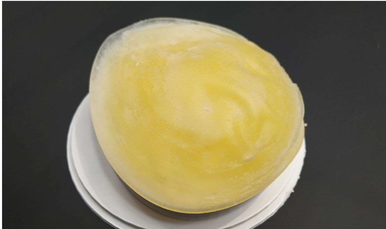
Figure 6.55. Printed full-scale prosthesis.
