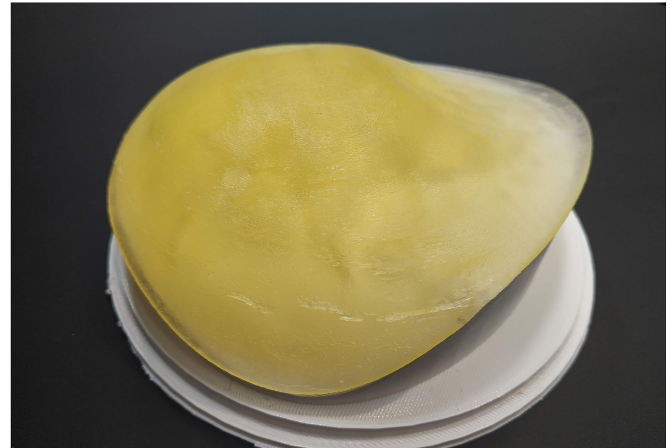
Figure 8.4. Flaws due to delamination in the final prototype.
