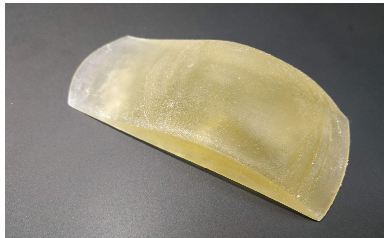
Figure 6.42. Prototype of a slice of a full-scale breast prosthesis for the Conclusive prototyping phase 2.
