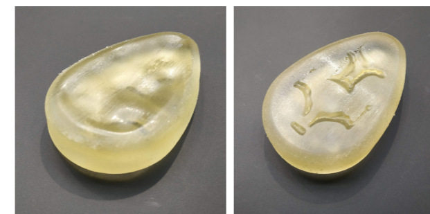
Figure 6.17. Teardrop-shaped sample. The testing surface is 0.6 mm thick and is printed on the bottom to ensure that the print will not fail due to its thinness. The image on the bottom left shows the testing face. The image on the bottom right shows the top cover (in the printing position), which is 3 mm thick. Flaws are visible in the parts that were horizontally printed on top of the gel-liquid mixture. Even if flaws are present, the material fully enclosed the inner mixture.
