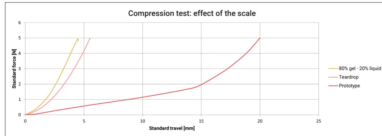
Figure 6.19. Compression test: effect of the scale.
