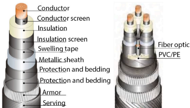
Fig. 1. Typical configuration of power cables.
