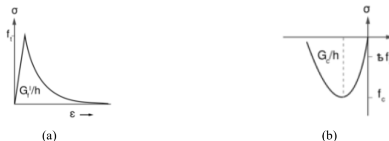
Figure 2. Masonry constitutive model, (a) represents the tensile and (b) the compressive behaviour
