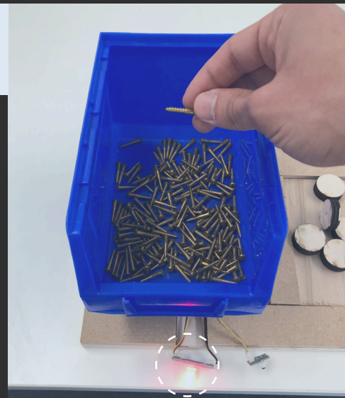
Figure 5.18: High precision of load cells testing with nails
