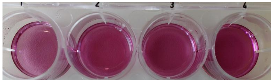
Figure 44. MTT Test Samples of 15 (1), 30(2), 60mg (3) of Cross-Linked Gelatin and 30mg of Plain Gelatin (4)
