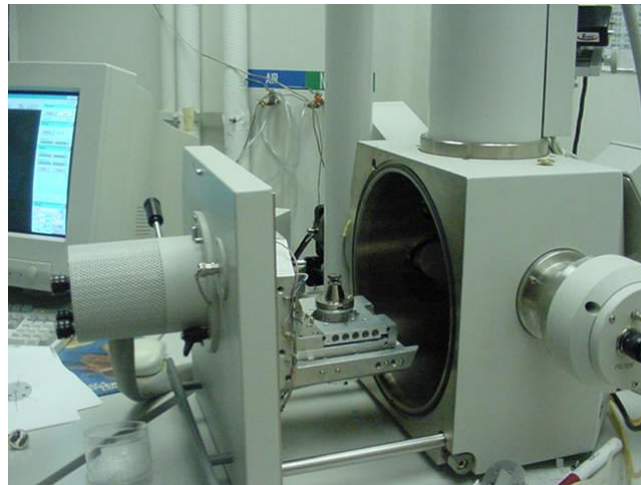
Figure 12. Scanning Electron Microscopy Equipment (Quanta 200F FEI) used for Particle Characterization
