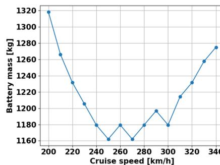
**Figure 12.8:** Resulting battery mass for varying cruise speeds.
