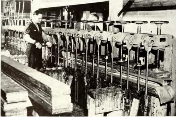
Figure 21.3: Gluing of flat laminated stock [57]
