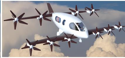
**Figure 7.2:** Aircraft in transition mode.
