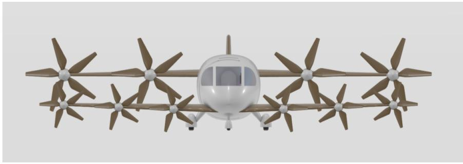
**Figure 17.7:** Front view of the final aircraft assembly in horizontal flight mode.
