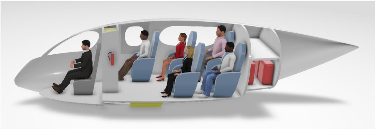
**Figure 8.5:** Right half of the outer fuselage surface including the windows, the emergency door and the interior, including the floor, walls, seats, luggage (red), fire extinguisher, battery packs (yellow) and mannequins for reference.
