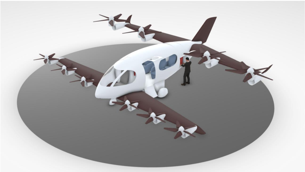
**Figure 17.10:** Perspective view of the final aircraft in VTOL flight mode with the entrance door and left luggage hatch opened, while the pilot is placing the luggage.
