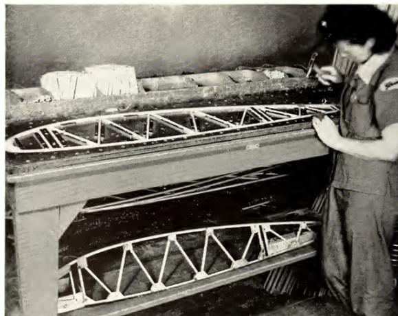
Figure 21.5: Manufacturing of wooden aircraft ribs using nail gluing [57]
