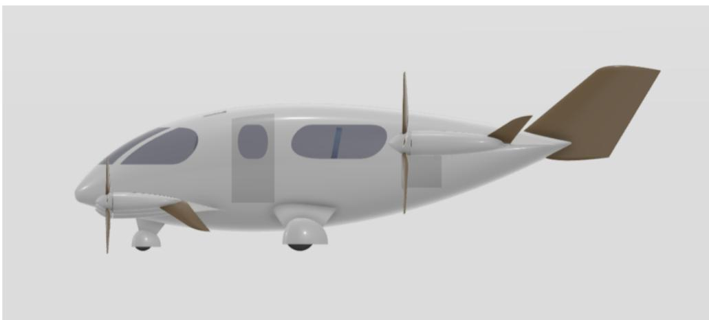
**Figure 17.6:** Side view of the final aircraft assembly in horizontal flight mode.
