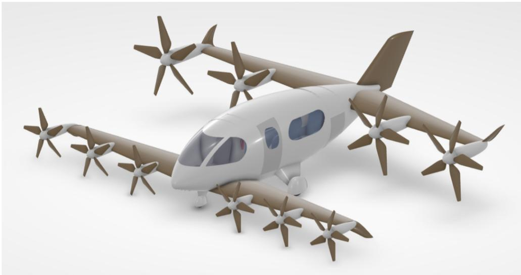
**Figure 17.5:** Isometric view of the final aircraft assembly in horizontal flight mode, including passengers and pilot.
