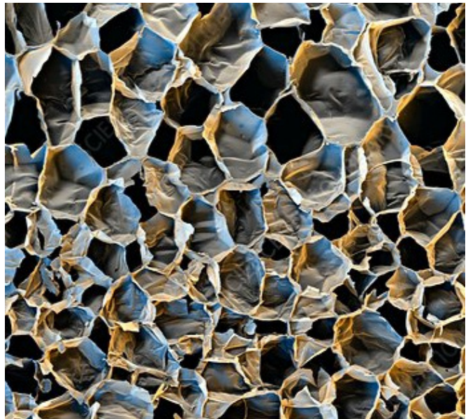
Polystyrene foam under a microscope. Credit: Stefan Diller/Science Photo Library.
