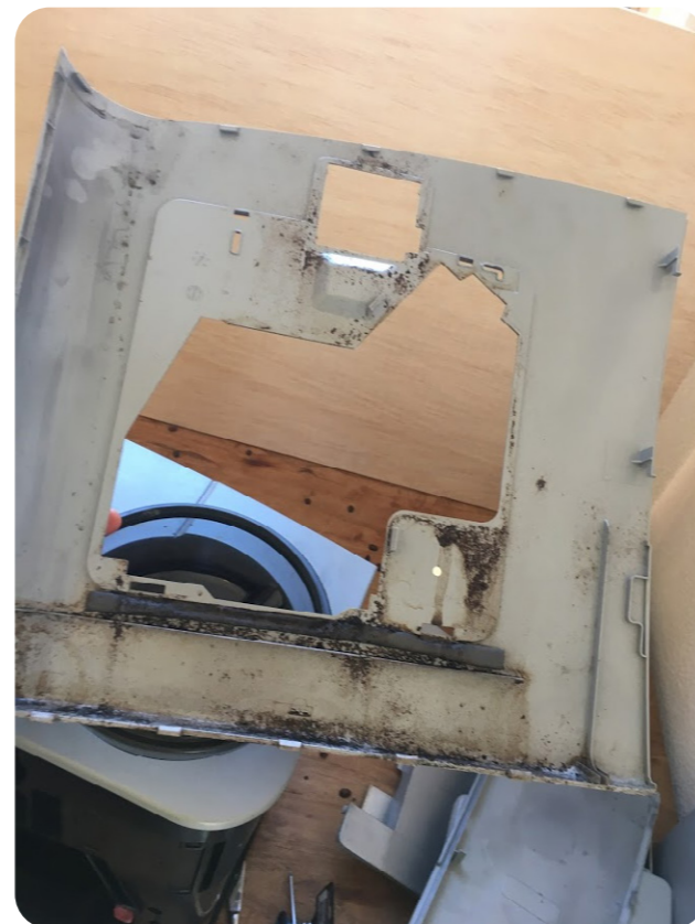
Figure 27: Dirt behind housing
