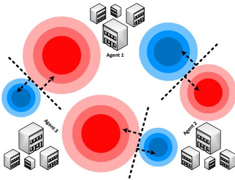
**Figure 2: Idealized three-building ATES case study.** Each building has a single ATES system which consists of a warm and a cold well. Warm and cold wells are shown with red and blue circles. The unwanted mutual interactions between ATES systems are shown via black dashed lines. Figure is taken from [10].
