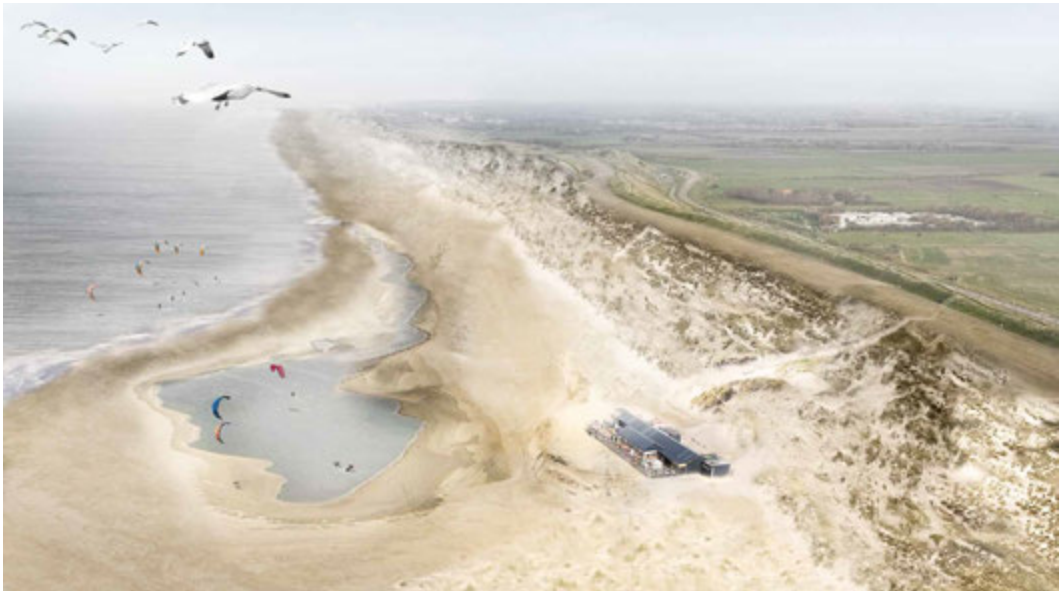
Design study phase 1: visualisation of a BwN-based mega-nourishment and new dune massive replacing the sea wall of Walcheren, with opportunities for beach recreation.
