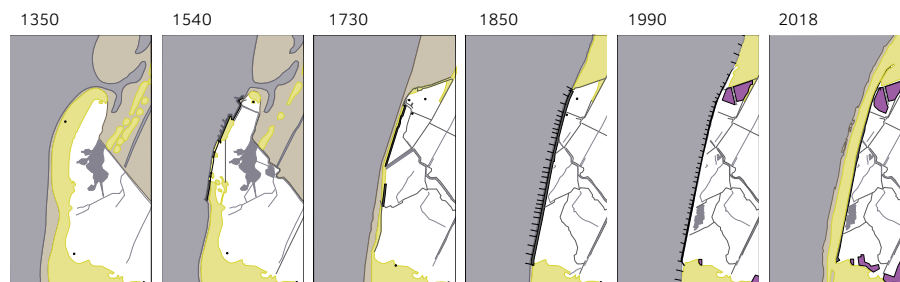
FIG. 4.27 Morphogenesis of the coast of Petten from an open tidal inlet system (1350, left) into a closed seawall (1850). In 2015, the seawall was replaced with a mega-nourishment, re-engineering the defence line back to the sandy system of before 1730. Images by the author, adapted from H. van Zijl.
