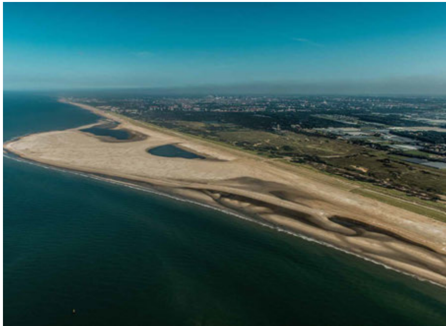
FIG. 1.6 Aerial photo of the Sand Motor, a Dutch mega-nourishment pilot in action (2012). Source: Rijkswaterstaat / Joop van Houdt.
