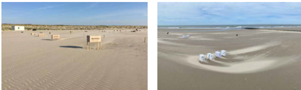
FIG. 1.13 Two examples of fieldwork carried out under the umbrella of the ShoreScape project: on the left, the testing site at the Sand Motor (2019), where the sedimentation patterns of beach housing on poles were tested; on the right, a field test at Vlieland beach (2020) investigating the tail pattern of row housing with a 45° dominant wind direction. Images by the author.
