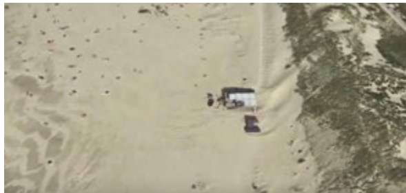
FIG. 3.56 Example of downwind tail development behind an elevated pavilion and non-elevated houses at Hargen, North Holland. Source: K. Wijnberg, UT, 2021.
