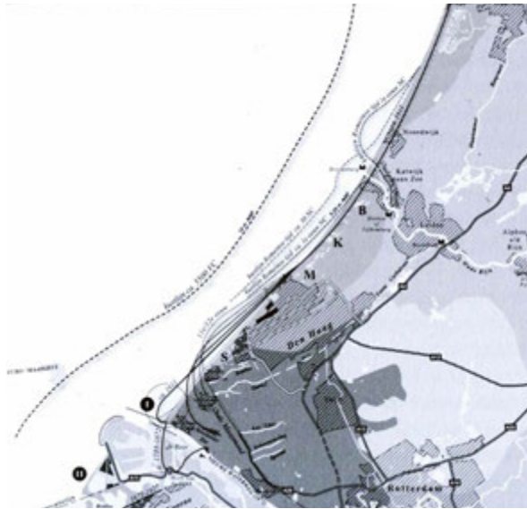
FIG. 4.48 Morphogenesis from the Meuse inlet from 1100 AC onwards, showing its southward movement as well as the coastal erosion of its former banks. Source: R. Waterman/De Ontwerpers, 2005.
