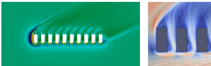
FIG. 1.14 Examples of CFD modelling of beach row housing: left the potential erosion and deposition patterns around beach row housing and right the nearbed wind field (speed and direction) Source: P. Pourtemouri, ShoreScape, 2021.
