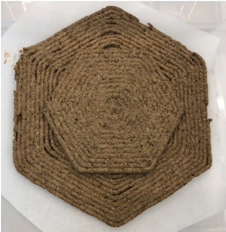
Figure 65 Acoustic panel with custom design on top
