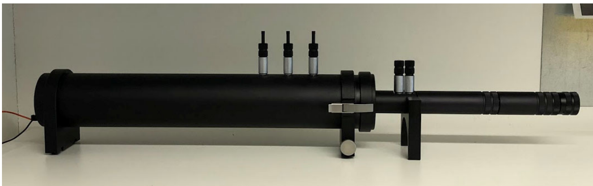
Figure 39 Impedance tube with the high frequency tool
