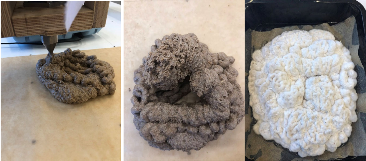
Figure 35 Test 1 Before and after growth
