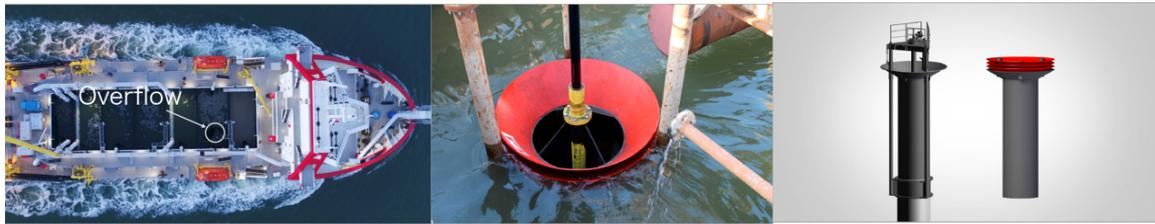
The overflow is positioned in the cargo. The soil of mixture sucked up would sink down. The operator can drain excess water on top by lowering the overflow.
