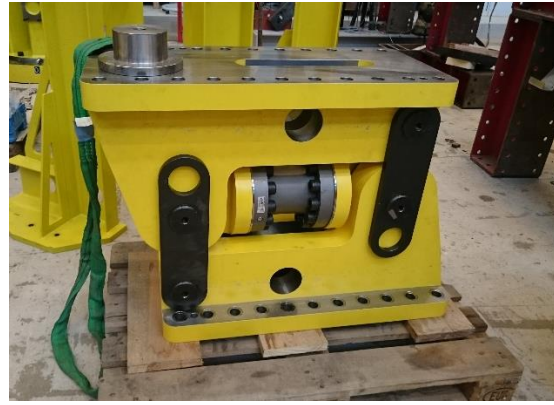
Figure 3.5: Specially designed calibration device for the load cell
