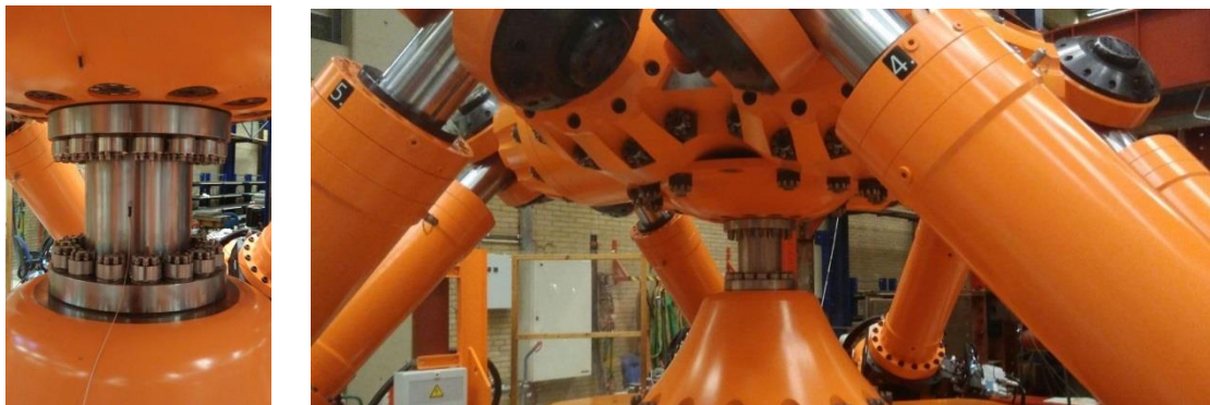
Figure 3.8: Detailed view of the mounted specimen (left), Overview of the test specimen mounted in the hexapod between the two bell-shaped interfaces (right)
