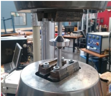
Figure 4.2: Test setup showing the bar specimen clamped in a uniaxial MTS fatigue test bench
