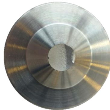
Figure 4.4: Fracture surface of a failed bar specimen with artificial defect
