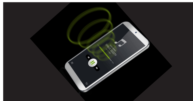
Figure 24. Redux ST is able to simulate buttons and play audio with their piezo actuated displays.
