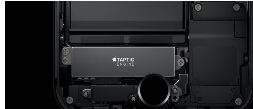
Figure 28. To deliver haptic feedback, Apple uses their proprietary taptic engine for all their devices. The Taptic Engine is a Linear Resonance Actuator.
