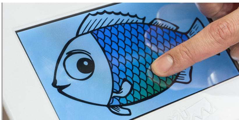
Figure 23. Hap2U demo where the user can feel the texture of the fish.
