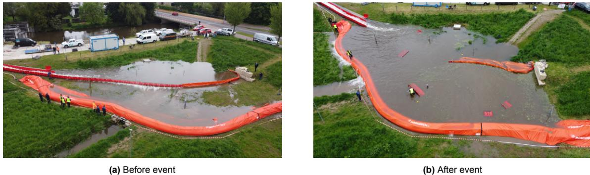
**Figure 1.3:** A visualisation of failure occurred during the experiment that took place in Roermond
