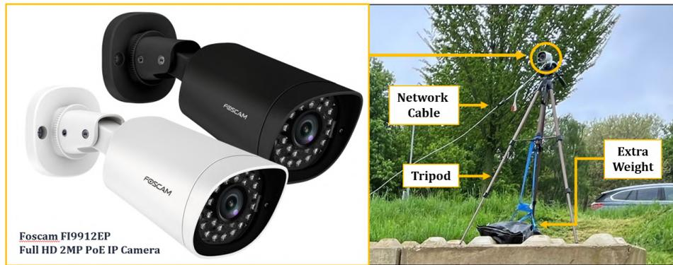
Figure 3.5: IP camera information and setup
