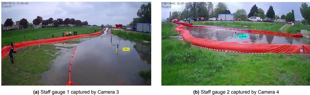
**Figure 3.14:** Visualisation of water level measurement in Kinovea
