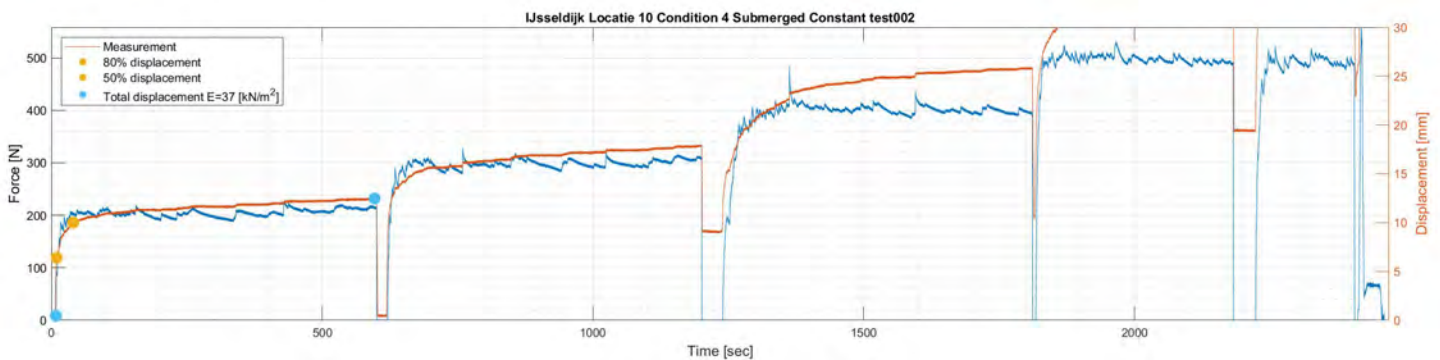
Displacement rate under step increased constant loading. The blue dots indicate the total or final displacement as result of the induced load during the first 600 seconds of loading. The yellow dot indicates 80% of the final displacement
