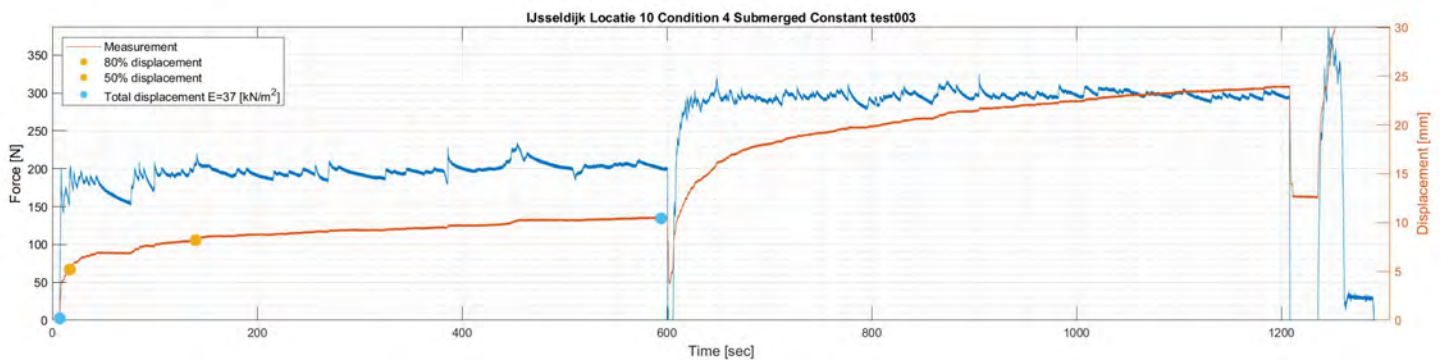
Displacement rate under step increased strain constant loading. The blue dots indicate the total or final displacement as result of the induced load during the first 600 seconds of loading. The yellow dot indicates 80% of the final displacement
