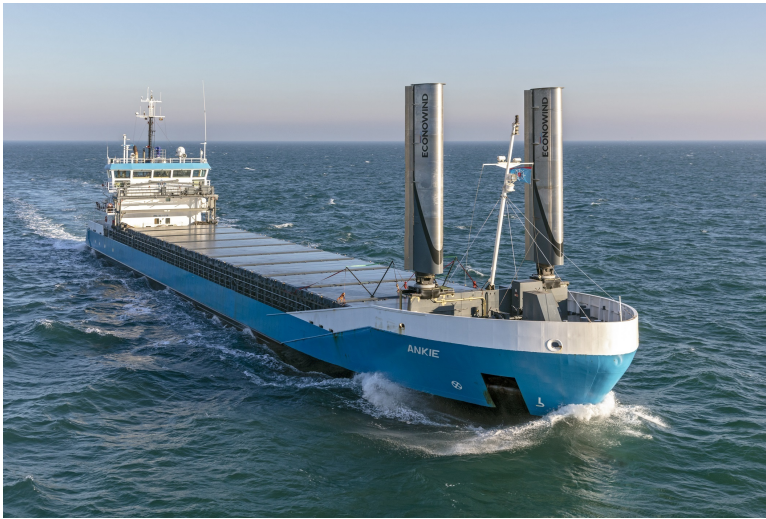
Figure 2.10: Suction wings application[52]
