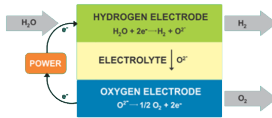
Figure 2-4: Representation of SOEC reactions [3].
