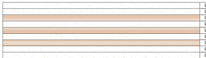
Figure 3.8. Layup CLT top view [0/0/90/0/90/0/90/0/0]
