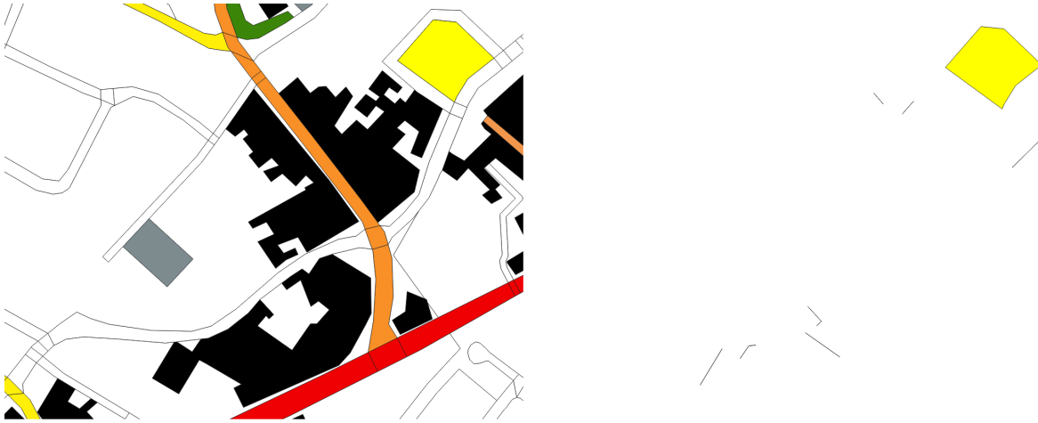
Figure 3.3: Examples of polygon which were not eligible to be processed by the current implementation. On the left, all objects are shown and on the right only degraded objects are visible (probably because of poor reconstruction of buildings). The yellow polygon was left for easier orientation.
