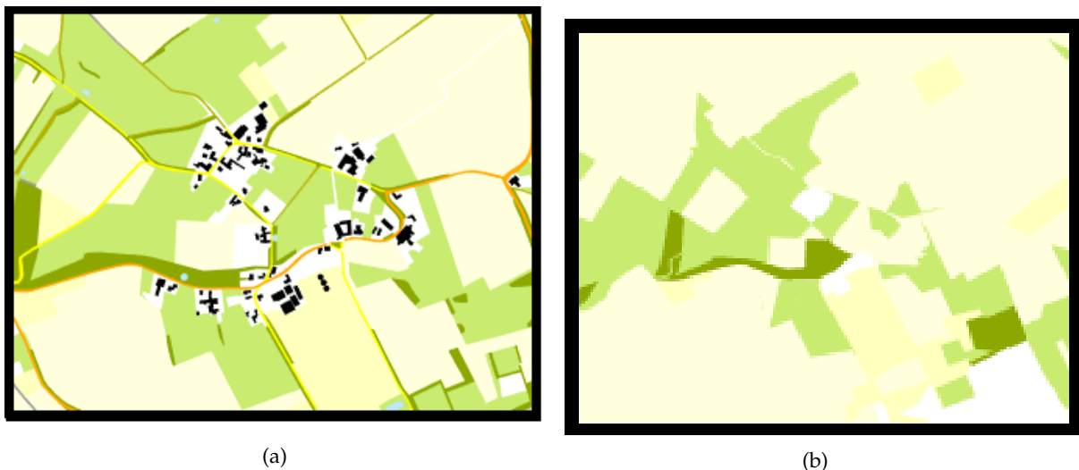
Figure 2.1: Comparison of maps presenting the same area at different scales. The map on the right is a result of generalization of the map on the left.
