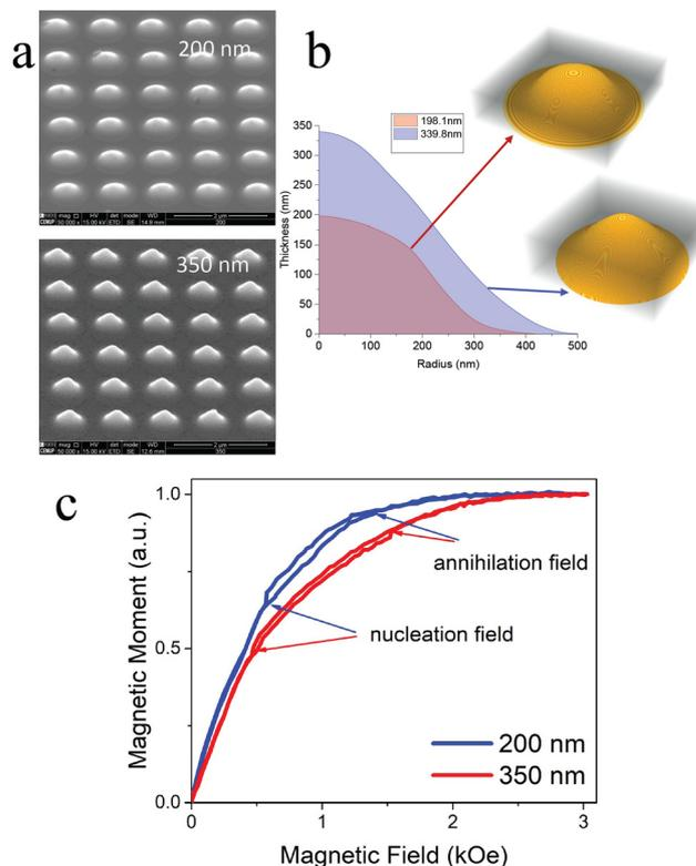
**Fig. 4** (a) Scanning electron microscopy images of 200 nm and 350 nm high nanodot arrays; (b) permalloy nanodot profiles derived from atomic force microscopy and renders of the model shapes of averaged nanodots for samples with 200 nm and 350 nm thick nanodots; (c) First quadrant of magnetization hysteresis loops for corresponding nanodot arrays. Nucleation and annihilation fields indicated with arrows.
