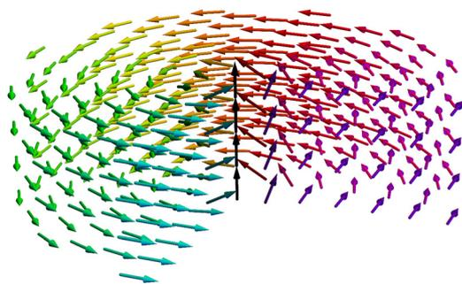
**Fig. 1** Cylindrical magnetic dot in the vortex state (not to scale), arrows represent spin momenta directions of individual spins in the cubic lattice. The color of the spins corresponds to the direction of the planar component of the spin, spins on the axis of the particle point out of plane and form the core of the magnetic vortex.
