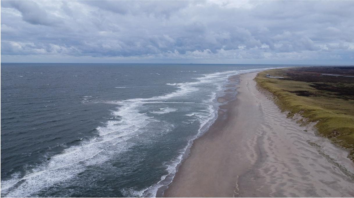
Figure 2.5: Bird perspective of the South West Texel coastline. In the middle of the photo there are a few horizontal lines in the water, which indicate submerged cross-shore groynes that get exposed only during low tides. The photo is taken at approximately JARKUS transect 900 and the coast bend starts at around transect 1000. The white single line of white-capping waves indicates that during these conditions the waves break only at 1 breaker bank.
