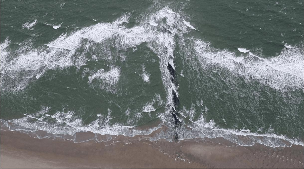
Figure A.5: Snapshot of waves arriving at the shoreline. This snapshot is taken during low water, when the cross-shore groyne is emerged. These groynes have a spatial distance of 400m.
