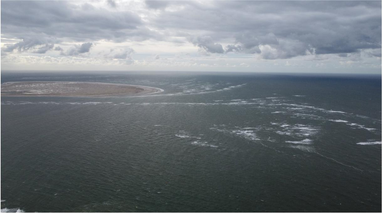
Figure A.3: Snapshot of waves coming from the NW. The whitecapping areas show the contours of the ebb tidal channel that is developing on the NUN.
